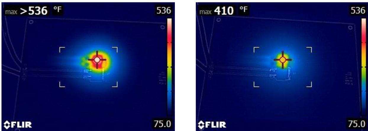
Left: Thermal signature of powered IC with 1 oz copper layer (approximately 35  $\mu$ m). Right: Thermal signature of powered IC with 25  $\mu$ m highly oriented graphite layer.
