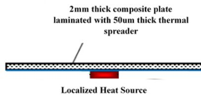
Above: Experimental design, Right: Thermal spreading comparison of 50 um thick copper (top right) and 50 um thick graphite (bottom right) yielding maximum spot temperatures of 59°C and 41.2°C, respectively.
