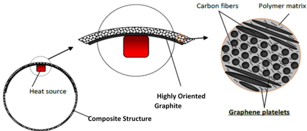
Schematic illustration of the proposed solution for in-plane thermal conductivity improvement. Highly thermally conductive graphene nanomaterials will be incorporated into the polymer matrix while a highly oriented graphite thermal spreader will be applied to the inner wall of the composite structure.
