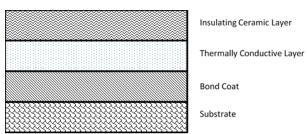
Stryke's innovative TBC architecture incorporates a thermally conductive layer to help rapidly dissipate heat from high flux environments.
